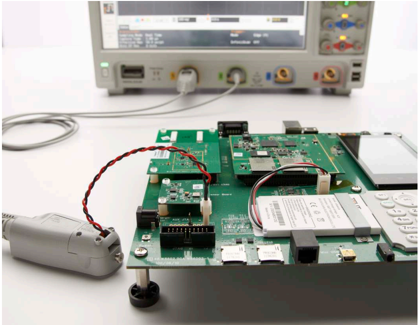
Figure 1. Keysight's ultra sensitive N2820A/N2821A current probes (with resolution as low as 50 \mu A) excel at measuring for small current levels typically found in battery powered devices.
